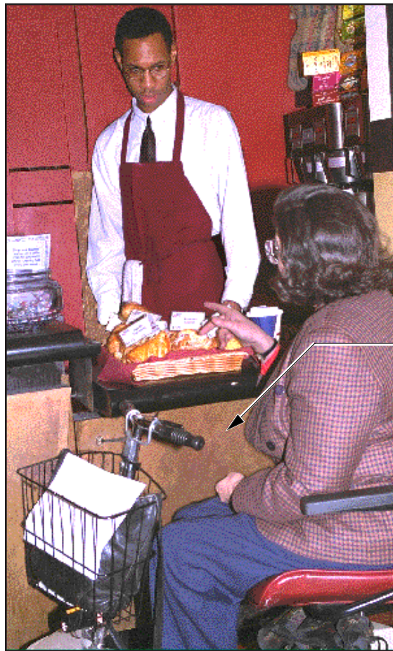
Lowered serving counter provides an accessible space to select and receive food items
